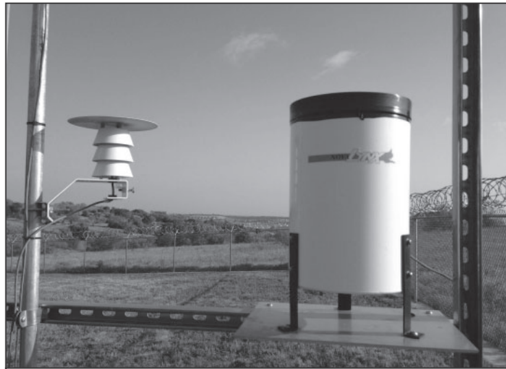
Tipping Bucket Used to Measure Rainfall
